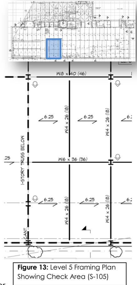
**Figure 13:** Level 5 Framing Plan Showing Check Area (S-105)
