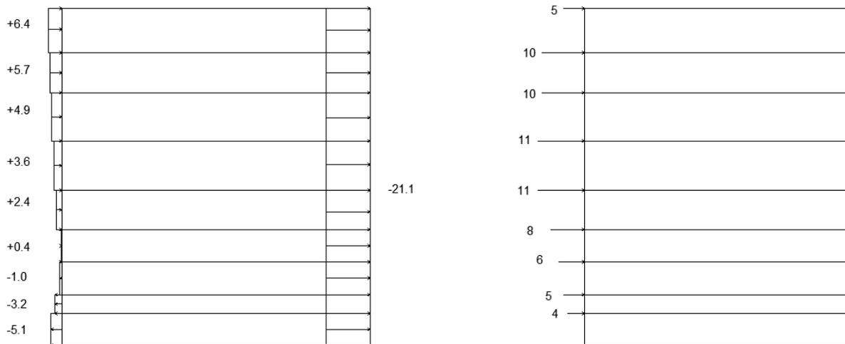
**Figure 17:** Pressures and Equivalent Lateral Forces
