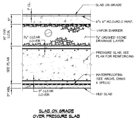
**Figure 4:** Pressure slab detail (S-201)
