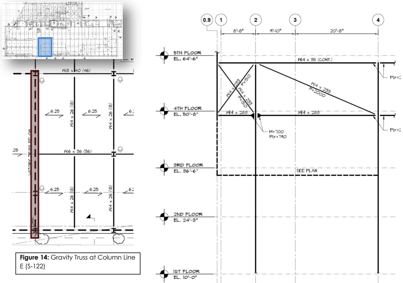
**Figure 14:** Gravity Truss at Column Line E (S-122)
